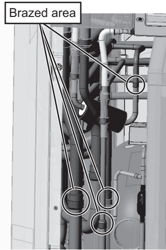
Removal of the front heat exchanger on a high-efficiency model (Figure 8)
